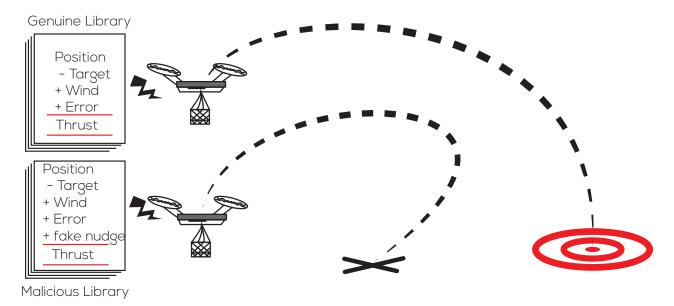
Robotic Vehicles could be effectively attacked in a manner that is undetectable by inserting malicious code into software libraries.
